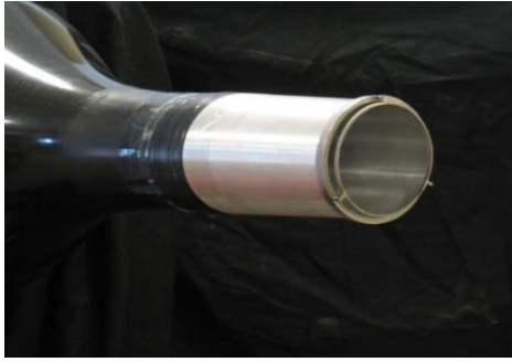
Figure 1. Views of the exit nozzle (upper figure) and the passive ring placed in the shear layer (lower figure).
